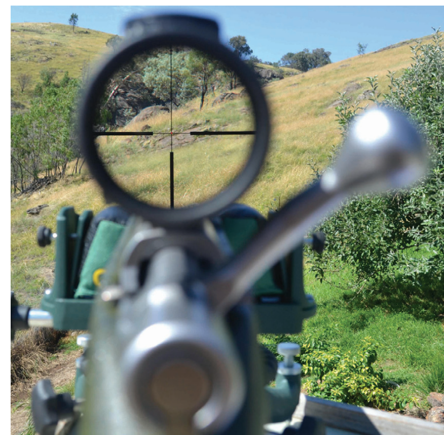
WINDAGE ADJUSTMENT DRUM. WINDAGE AND ELEVATION ARE ADJUSTED IN 7MM CLICKS, AND THE DRUMS PULL OUT FOR SETTING.
