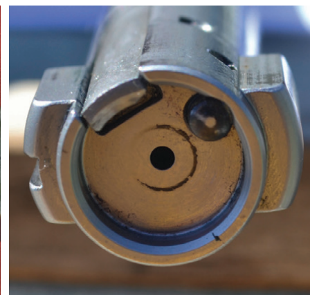
BOLT FACE SHOWING PLUNGER EJECTOR AND EXTRACTOR CLAW.
