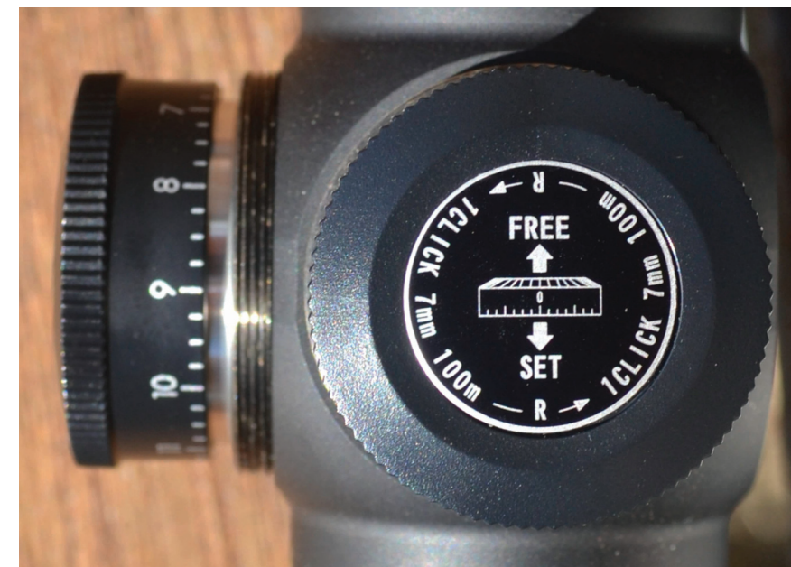
WINDAGE ADJUSTMENT DRUM. WINDAGE AND ELEVATION ARE ADJUSTED IN 7MM CLICKS, AND THE DRUMS PULL OUT FOR SETTING.
