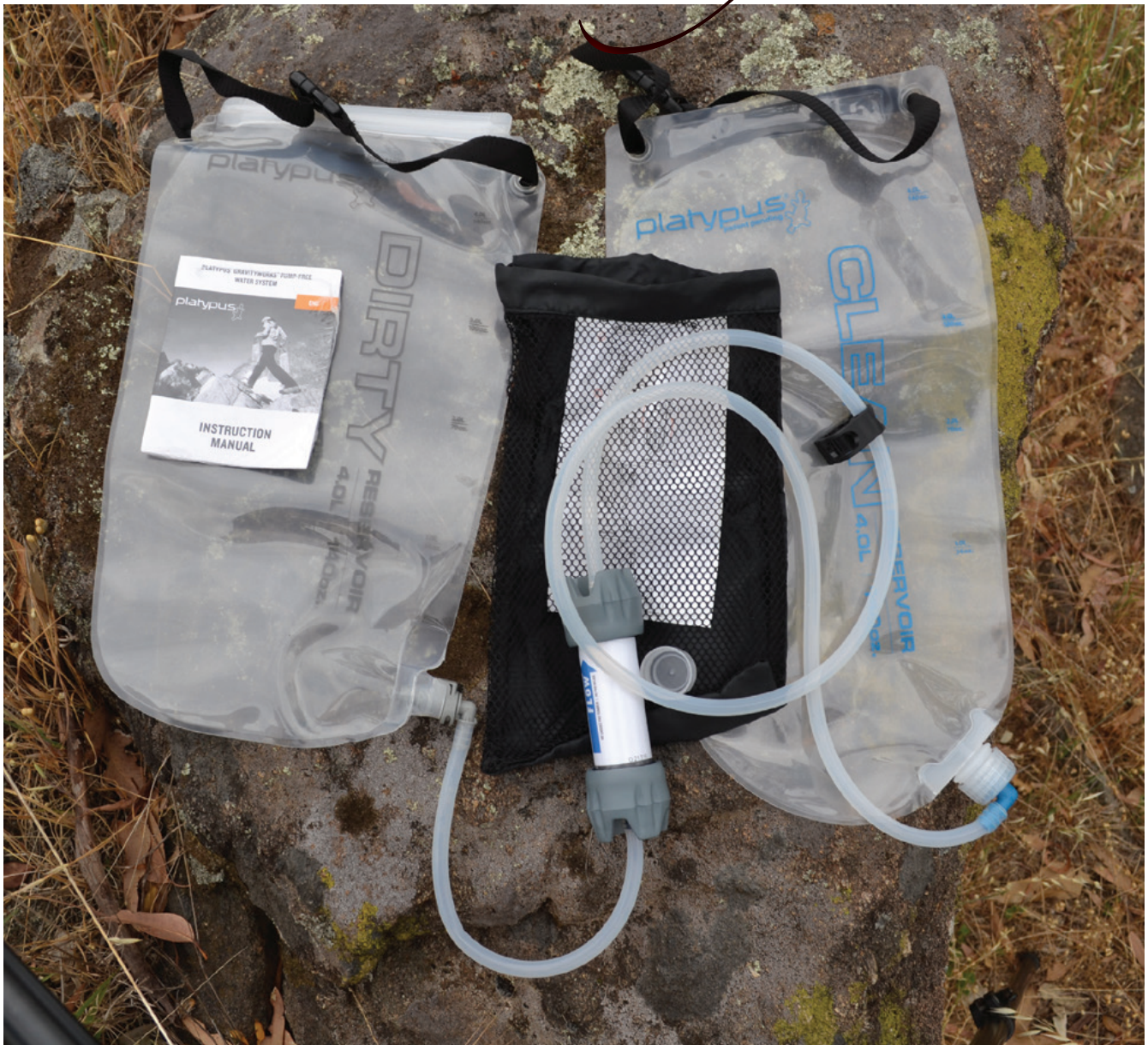
The component parts – on the left is the "Dirty" water bag and the instructions. The "Clean" water bag is on the right. The filter, 300mm dirty hose, 1220mm clean hose, black plastic shutoff clamp and "clean side cap" are on top of the nylon storage bag.
