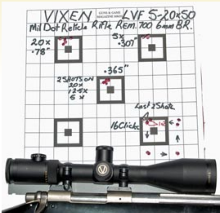
(Above) The 5-20x50 test target shot with the 700 Remington in 6mm BR. Perhaps the 6 shots consisting of 2 shots each on the highest, lowest and middle power all going into 0.365" says it all. The round the target test of 64 clicks to give an almost perfect result. The group shot on 5 power ain't half bad either! (Right) The 2.5-10x50 test target with the sort of results some of the expensive scope manufacturers would be envious of. The very slight shift in the 2 x 5-shot groups from 10 to 2.5 power is more than likely the method I use to obtain a reasonable hold on the low power. The reticle intersection covers over 2" at 100 yards so it is very difficult to keep a consistent hold on the aiming mark. I use in this case the top bull and the left hand bull to help me centre the cross in the same place shot to shot as the bulls can be just seen either side and above and below of a single wire. (Below) The author fitting the Vixen scopes using a Buffalo River cleaning aid as a cradle. This is the bench the test targets were shot from.
